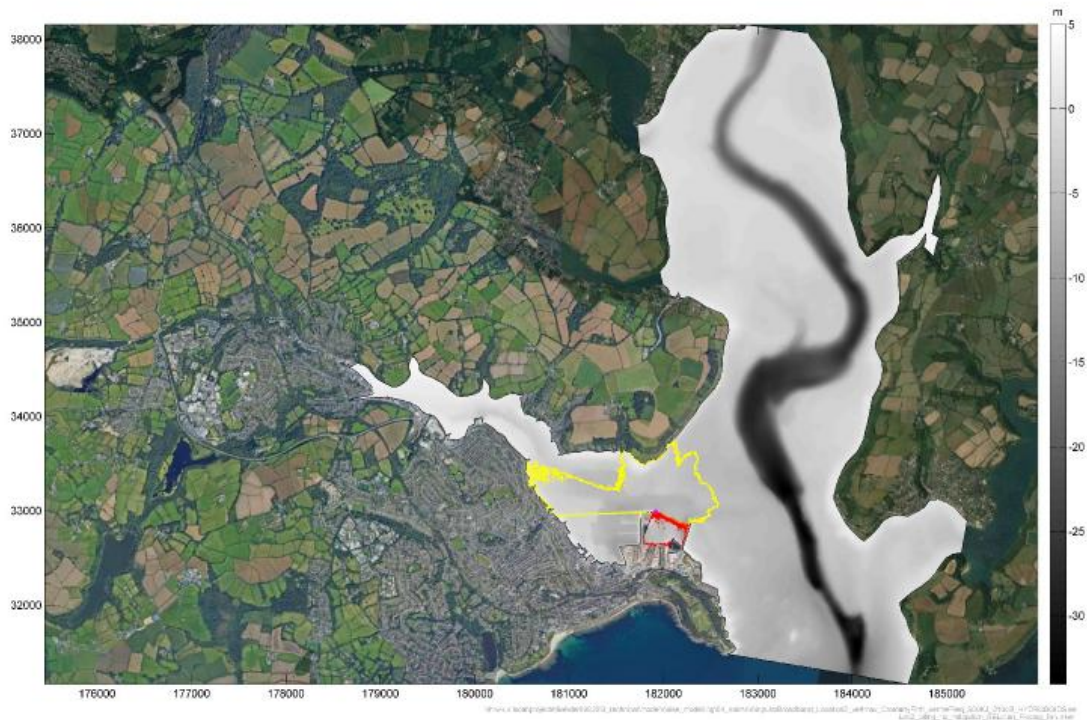
Figure 7. Predicted SELcum impact footprint for fleeing fish for percussive piling, with a soft start procedure, at the Western Wharf (Location 2).
