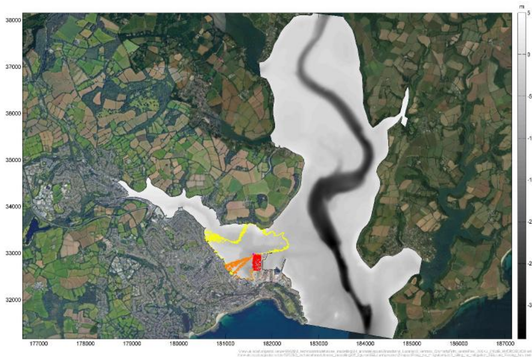
Figure 8. Predicted SELcum impact footprint for fleeing fish for percussive piling, with a soft start procedure, at the Queen's Wharf (Location 3).
