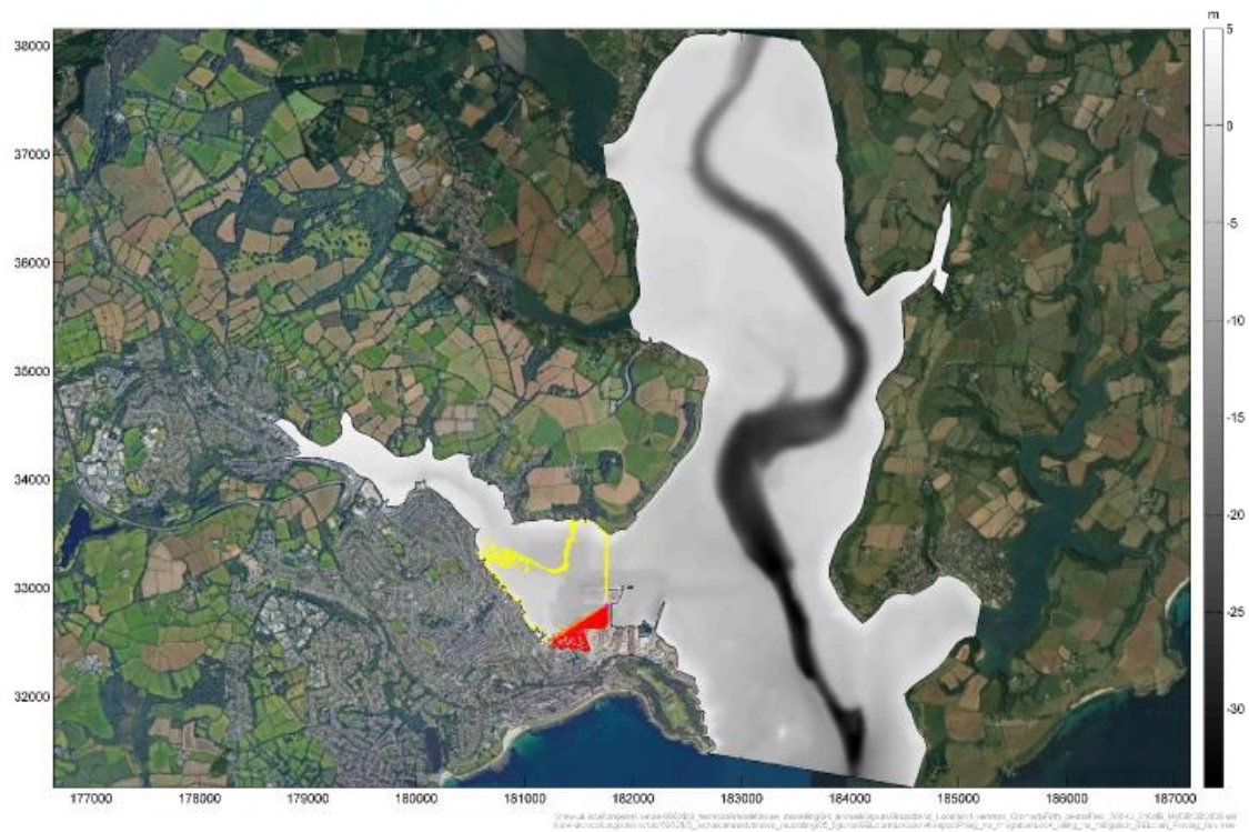
Figure 9. Predicted SELcum impact footprint for fleeing fish for percussive piling, with a soft start procedure, at the FLOW Deck (Location 4).
