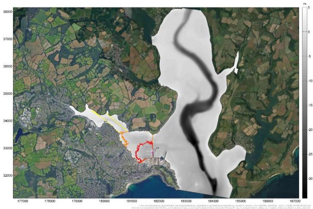
Figure 5. Predicted SELcum impact footprint for the for category 2 stationary fish for percussive piling, with a soft start procedure, at the FLOW Deck (Location 4).
